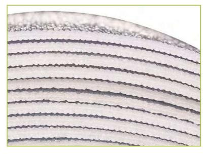
Consists of a variable-width layer of closed microcell polyethylene foam sandwiched between two layers of aluminum foil or one layer of film and one layer of aluminum foil.
